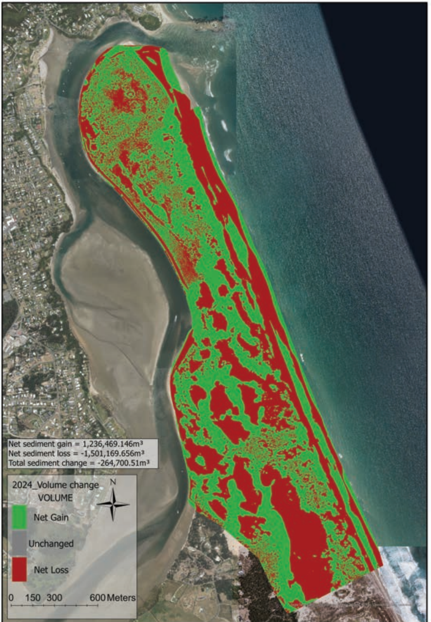
Figure 6. Cut-and-fill analysis to evaluate the net gain and loss of sand (2018 v 2024)
